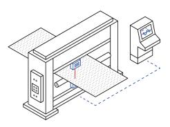
The measurement is carried out on a vertical basis across the cloth by an X-ray transceiver on a carriage that continuously moves from one extreme of the cloth to the other extreme.
